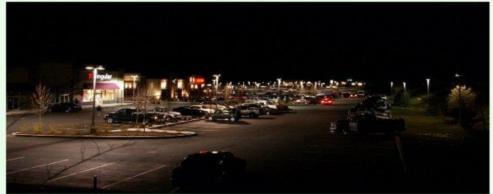
Fully Shielded parking lot lights
