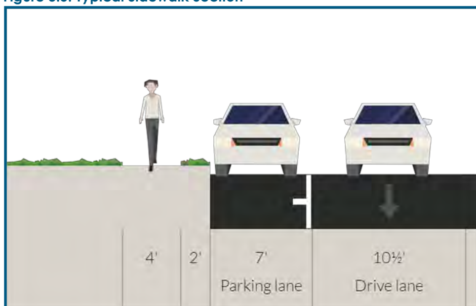
Figure 3.5: Typical Sidewalk Section
